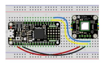
Board 3V to sensor VIN (red wire)
