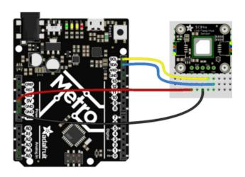
Connect board VIN (red wire) to Arduino 5V if you are running a 5V board Arduino (Uno, etc.). If your board is 3V, connect to that instead.
