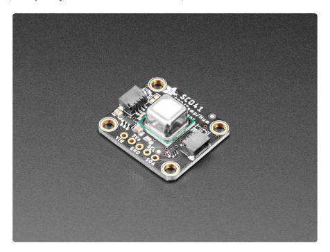
Compared to the illustrious SCD-30 (http://adafru.it/4867), this sensor uses a different measurement technique, which allows it to be much smaller. The overall data quality should be very similar, however. Like the SCD-30, this sensor has data read over I2C, so it works very nicely with just about any microcontroller or microcomputer. There's both Arduino and Python/CircuitPython code so you can get started in a jiffy.
