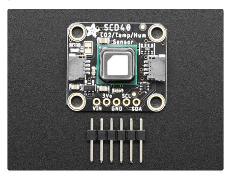
The SCD-40 and SCD-41 are photoacoustic 'true' CO2 sensors that will tell you the CO2 PPM (parts-per-million) composition of ambient air. Unlike the SGP30, this sensor
