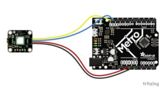
Connect **board VIN** (**red wire**) to **Arduino 5V** if you are running a **5V** board Arduino (Uno, etc.). If your board is **3V**, connect to that instead.
